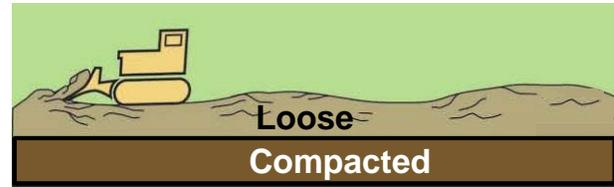
**Diagram 1.** End-dumping and final grading on a truck-and-haul surface mine. Subsurface materials have been placed as described in the permit and have been compacted by equipment operations. Surface materials are dumped over the compacted subsurface to a depth of 4 to 6 feet (upper) and are graded only lightly so that they remain loose and uncompacted (lower).
