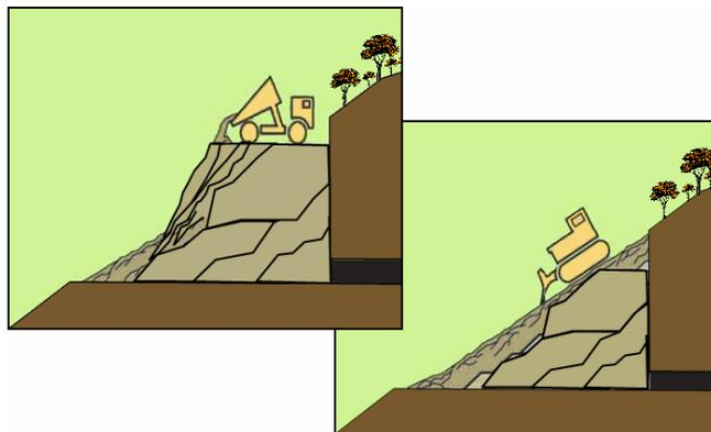
**Diagram 4:** Soil placement and final grading on a steep-slope contour mine where the backfill is constructed of approved topsoil substitute material and does not require compaction to maintain stability. The material is dumped in place (left) as per normal practice and then struck off to shape the backfill (right) but not graded smoothly. The dozer grades downward and trams back up on roads or defined tramways so as to minimize tracking back over materials that have already been shaped.
